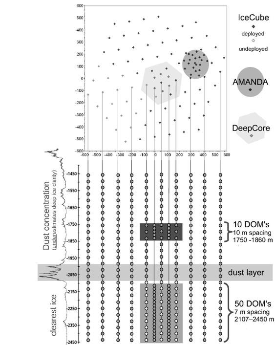
Fig. 1. Schematic view of the IceCube DeepCore
